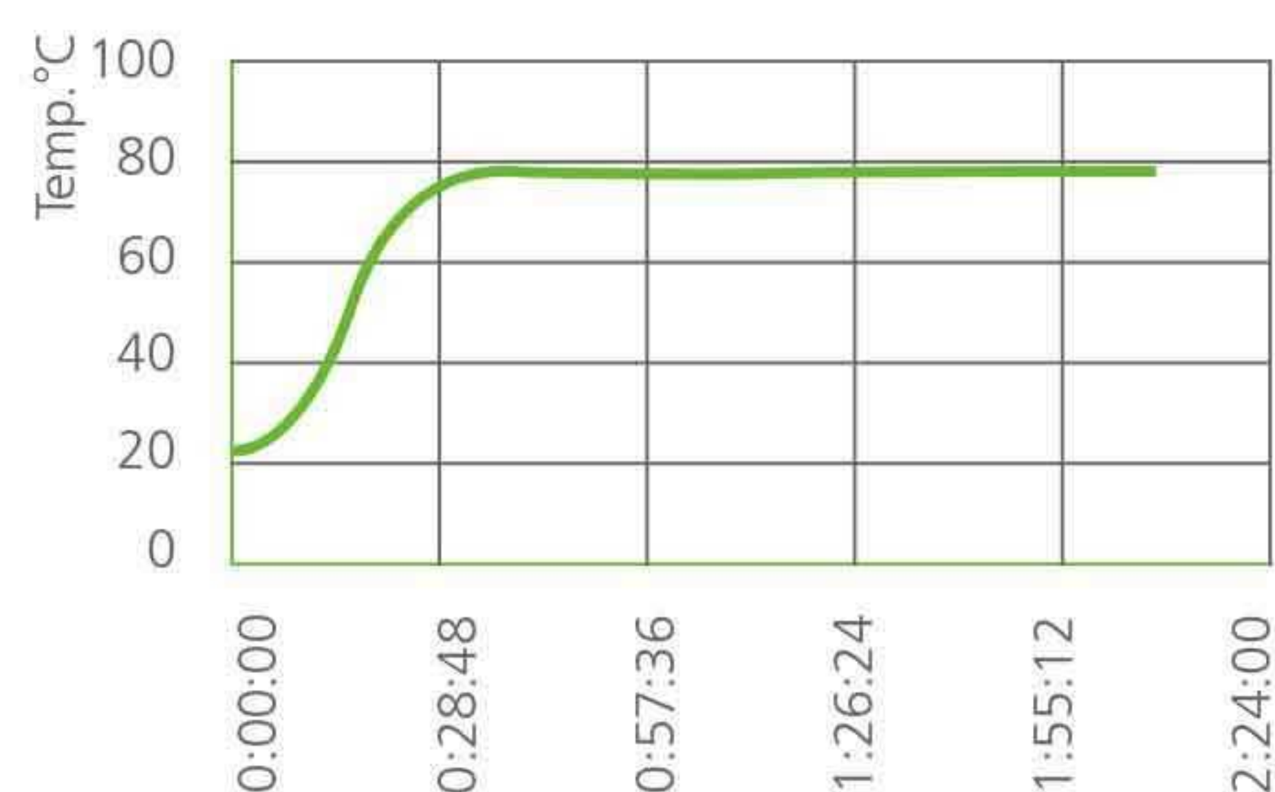
250ml water heated up to 80°C (MS-H-ProA)
